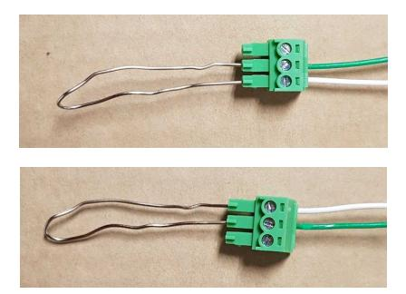
To demonstrate, if the lock mechanism is unengaged (unlocked) before you connect in the paperclip, it should be engaged (locked) after you connect the paperclip.
