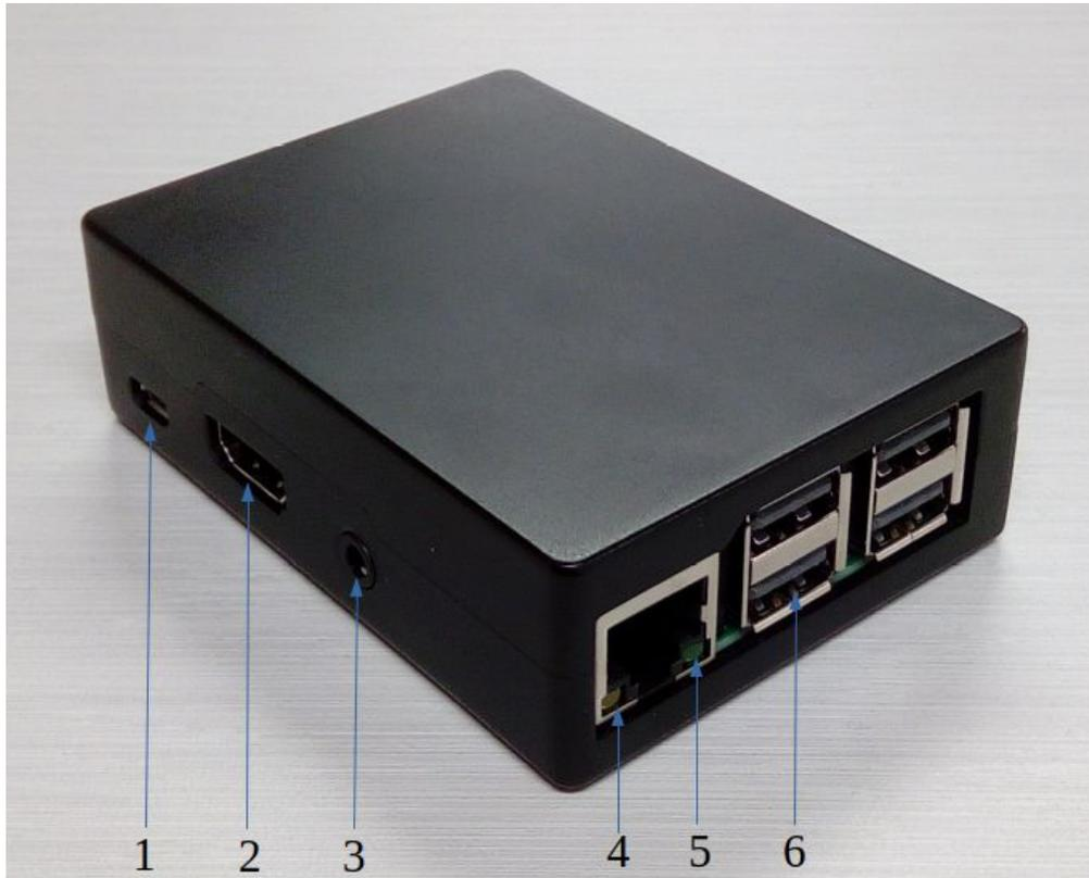
The GateKeeper Mini (GK-Mini) is a stand-alone mini-computer, similar to the GateKeeper, but designed to handle desktop readers, receipt printers, and other functions. It is not designed to control magnetic locks on doors.
