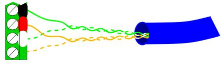
The other conductors in the cable (not shown) can be connected to the relay terminals to opeate the lock circuit.
