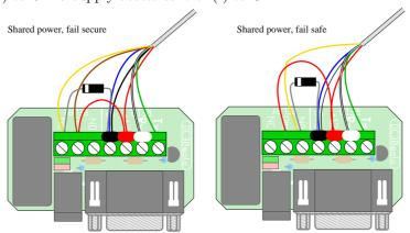
Note: the brown wire only used for fail safe with exit button
