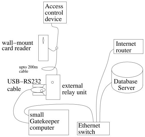
These RFID reader do not contain a relay to activate the access control, instead an external relay unit is used which connectes to the gatekeeper using a USB to RS232 cable. Power supplies not shown.
