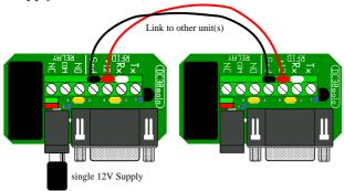
Alternatively the power supply can be connected to the screw terminals instead of to the socket
