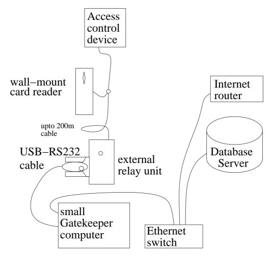
These RFID readers do not contain a relay to activate the access control, or connect to the LAN. Instead an external relay unit is used which connects to the gatekeeper using a USB to RS232 cable and also passes the RS232 signals through to communicate with the reader. Only one reader is shown, but several can be connected, i.e. by using multi-end cables or USB hubs.
