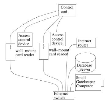
These RFID readers connect via ethernet LAN cables to a network switch instead of connecting directly to the server.
