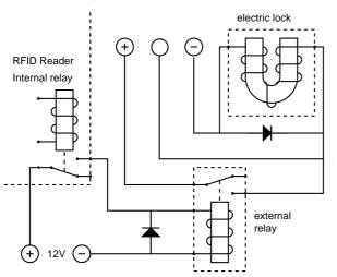
For locks that require power to unlock the external relay contacts should be wired parallel to the other unlocking switches Remember to fit diodes, failure to do so may lead to the RFID reader quitting.
