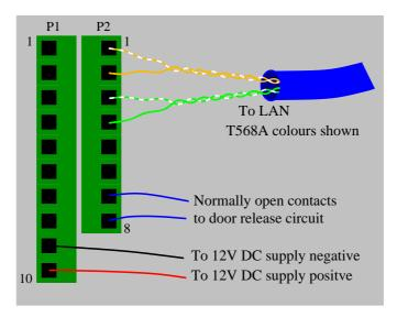
This image shows the connectors on the rear of the reader connect the LAN and the door circuit as shown.
