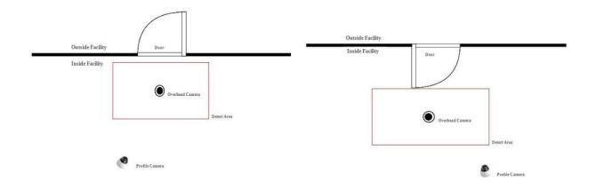
Figure 1 & 2: Difference in overhead camera position when the opening door obstructs the
