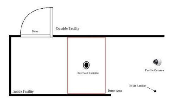
Figure 3: Position of overhead camera with narrow passageway
