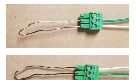
To demonstrate, if the lock mechanism is unengaged (unlocked) before you connect in the paperclip, it should be engaged (locked) after you connect the paperclip.
